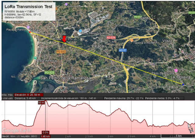
Fig. 4. Elevation profile and distance achieved in LoRa mode.
